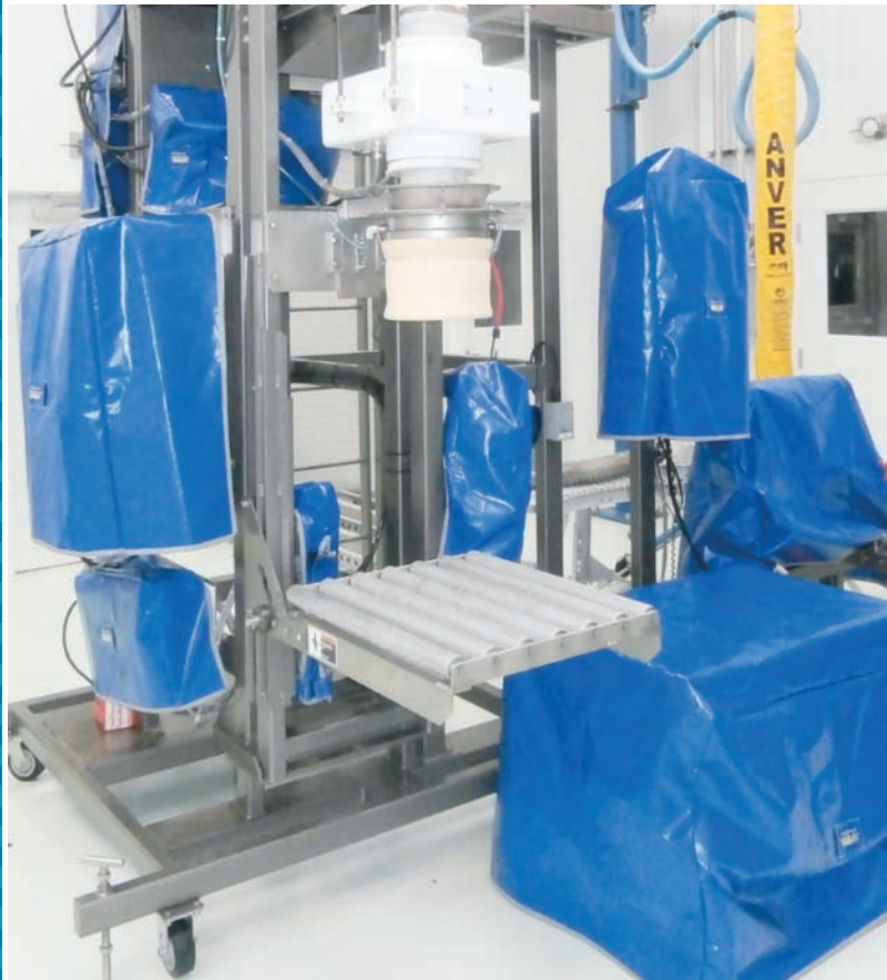
INSULTECH® Rain Shield is custom designed for each device. Easy on and easy off, removable and reusable.
